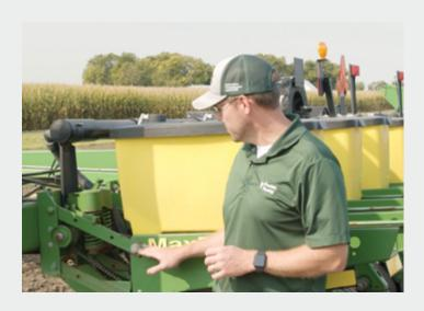
There are many different options available for you when you're doing parallel arm maintenance on your planter, including new OEM components or aftermarket solutions, including kits from SI Distributing for parallel arms, or Highland Machining's replaceable bushing kit. Harvest International also has a complete parallel arms set.
